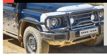
Provides extra protection for the fenders when off-road, rock crawling or from any other impact. (Roo Bar and Side Runners or Rock Sliders are required for fitment)
