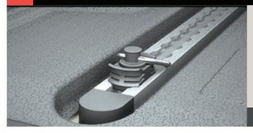
Utility rails fit into the floor of the rear compartments and allow for the secure fastening of loads and accessories. Quick release tie-down rings are required with this accessory.
