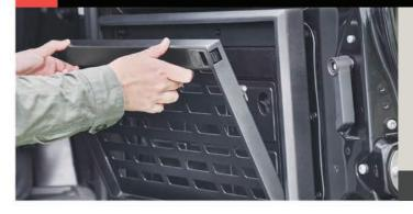
A smart feature with two uses: unfolded as a table and as a molle panel to secure pouches when in the upright position.
