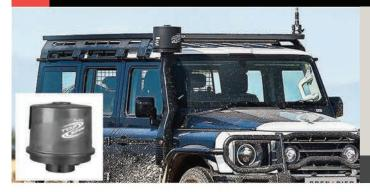
An additional filtering layer for the raised air intake. Provides the engine with cleaner airflow, keeping out dust and dirt by spinning the air as it enters the raised air intake, preventing contaminants from entering the intakeduct.
