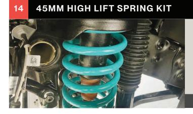
A spring lift kit raises the vehicle body and creates better ground clearance for use off road whilst giving a more muscular appearance. Also provides additional clearance when fitting larger wheel and tyre combinations.
