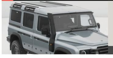
Raising the position of the engine air intake ensures the engine is fed with cleaner and cooler air in dusty environments.
