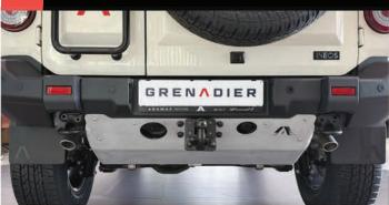
Heavy duty front and rear underbody protection with built in hitch receiver at the rear. Additional protection for the underbody area and improved ramp and departure angles when off- road.
