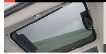
Unique to the Grenadier, these sunshades clip into the Safari Window aperture and reduce the sunlight and heat coming into the cabin. Easily fitted and removed and supplied in a zip up storage bag.
