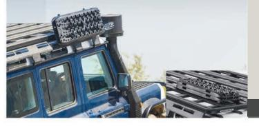
Allows you to secure sand ladders in flat position on the roof of your vehicle to avoid using up cabin space. Note: Requires a Roof Rack or Lader Rack.
