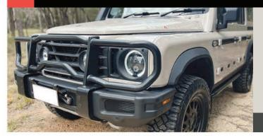
The Grenadier Roo bar provides protection from impact to the front grill, lights and bodywork of your vehicle. Made of high-quality material with a sleek and sporty design that will enhance the look of your vehicle. Additionally, provides mounting points for additional lights and is compatible with winch set up.
