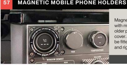
Magnetic Phone Holders can be used with most recent mobile phones or older phones fitted with a magnetic cover. A maximum of two holders can be fitted into your Grenadier on the left and right sides of the console.
