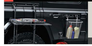
Quick release tie-down rings allow you to secure luggage or heavy loads to the utility rails on the sides and in the rear compartment floor of the vehicle.
