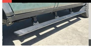
Electrically operated sidesteps extend and retract when the side doors are opened and closed. They are wired to an original switch in the Overhead Panel and can be switched off when driving offroad when greater ground clearance is required.
