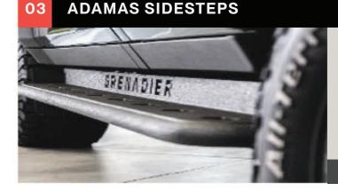
Sidesteps securely mounted to the chassis of the vehicle and make entry and exit much easier especially for children. Protected by a robust rubberised coating with "GRENADIER" laser cut into the step.
