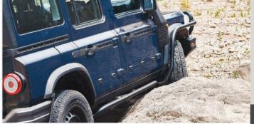
Additional protection for the body and chassis of your vehicle while off-roading. Made of heavy-duty materials and tested under the toughest conditions, the Rock Sliders can also be used as anchoring points for Hi-Lift jack.
